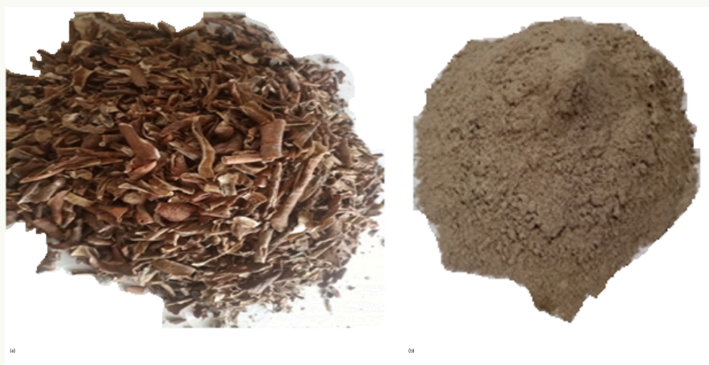
Figure 1: Cassava cortex preparation used in this study: (a) dried cassava cortex and (b) 150 µm sieved milled cassava cortex.
